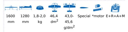
\*Motor: electro – AXI 2820/12, 3S LiPo 2,5 - 3,2Ah, propeller 12?6 Servos: HS-225 for ailerons, HS-325BB for elevator and rudder.
