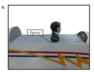
Position the canopy onto the fuselage. Trace around the canopy and onto the fuselage using a felt-tipped pen. Carefully cut and remove covering material from the fuselage where the canopy makes contact, exposing the bare wood. Then permanently glue the canopy in place with epoxy glue or special "canopy glue".
