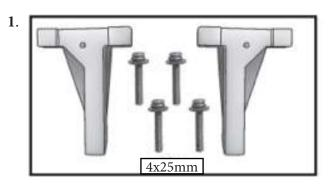
Use four 4x25mm head bolts and four 4mm washers to attach the engine mount rails to the firewall. Tighten the screws .Make sure to use threadlock on the screws to help prevent them from vibrating loose.
