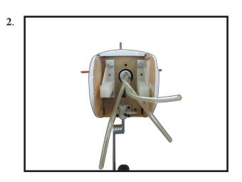
Position the engine with the drive washer (135mm) forward of the firewall as shown.
