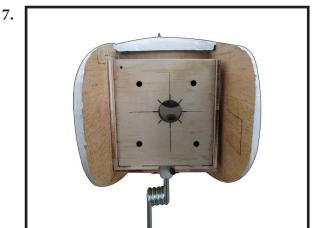
Attach the motor to the front of the electric motor box using four 4mm blind nut, four M4x16mm hex head bolts to secure the motor. Please see picture shown.
