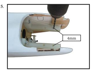
On the fie wall has the location for the throttle pusshrod tube (pre-drill).
