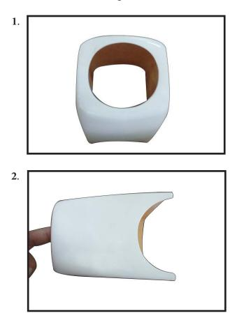
Tape the cowl to the fuselage using low-tack tape.
