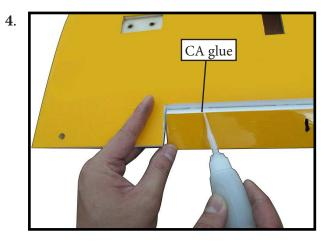
Turn the wing panel over and deflect the flap in the opposite direction from the opposite side. Apply thin C/A glue to each hinge, making sure that the C/A penetrates into both the flap and wing panel.
