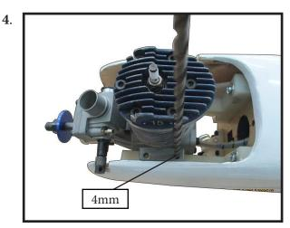
Use a drill to drill the four holes in the engine mount rails.
