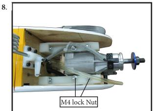
Reinstall the servo horn by sliding the connector over the pushrod wire. Center the throttle stick and trim and install the servo horn perpendicular to the servo center line.
