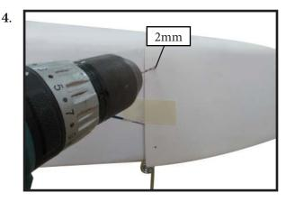
Install the muffler and muffler extension onto the engine and make the cutout in the cowl for muffler clearance. Connect the fuel and pressure lines to the carburetor, muffler and fuel filer valve. Secure the cowl to fuselage using the M3x10mm socket head screws.Putting a small length of silicon fuel tube under the head of the screw helps with vibration.
