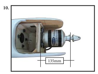
Attach the speed control to the sidem of the motor box using two-sided tape and tie wraps. Connect the appropriate leads from the speed control to the motor. Make sure the leads will not interfere with the operation of the motor.
