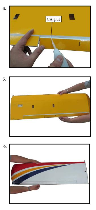
Turn the wing panel over and deflect the aileron in the opposite direction from the opposite side. Apply thin C/A glue to each hinge, making sure that the C/A penetrates into both the aileron and wing panel.
