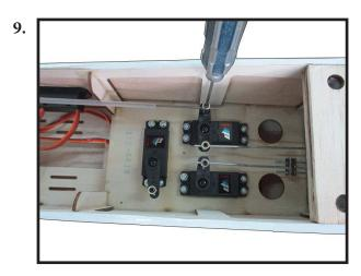
Move the throttle stick to the closed position and move the carburetor to closed. Use a 2.5mm hex wrench to tighten the screw that secures the throttle pushrod wire. Make sure to use threadlock on the screw so it does not vibrate loose. 10.
