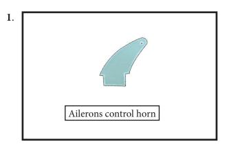
Use sandpaper to scuff the bottom of the aileron and flap control horns. Use a paper towel and isopropyl alcohol to remove any oils or debris from the control horns.
