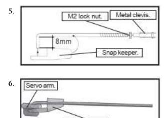
Connect the linkage as shown and secure the control wire with a snap keeper.
