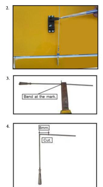
Make a 90-degree bend at the mark and cut off the excess wire leaving 8mm past the bend.
