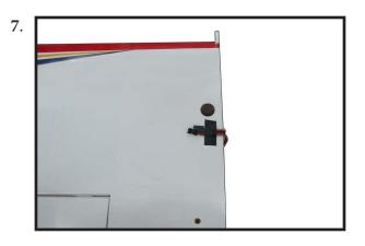
Reinstall the servo into the servo mount and secure the servo inplace using the wood screws provided with you radio system.
