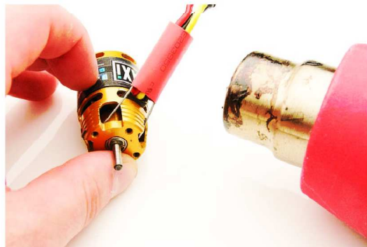
Nasuňte bužíрку na pružinku s kabely a horkovzdušnou pistolí smrštěte. Slide the tube onto the spring with the cables and shrink with a hot air gun.
