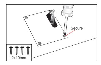
□ 5) Repeat the procedure to install the aileron servos in the opposite wing half.
