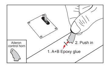
$\ \square$  3) Repeat the procedure to install the control horn on the opposite aileron.
