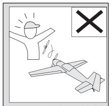
**ALWAYS** adjust the engine from behind the propeller, and do not allow any part of your body to be in line with the propeller.
