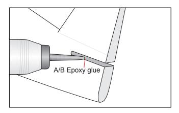
After the epoxy has fully cured, remove the masking tape or T-pins used to hold the stabilizer in place and carefully inspect the glue joints. Use more epoxy to fill in any gaps that may exits that were not filled previously and clean up the excess using a paper towel and rubbing alcohol.
