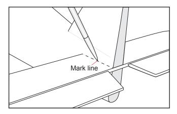
☐ 6) Remove the stabilizer. Using a modeling knife and ruler **CAREFULLY** cut 1mm **inside** the marked lines. Remove the covering from the top and the bottom of the tail plane.
