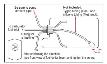
□ 5) Test fit the stopper assembly into the tank. It may be necessary to remove some of the flashing around the tank opening using a modeling knife. If flashing is present, make sure none of it falls into the tank.
