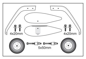
$\Box$  **1**) Assemble and mounting the wheel pants as shown in the following pictures.
