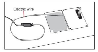
□ 4) Place the servo into the servo tray. Center the servo within the tray and drill 1.5mm pilot holes through the block of wood for each of the four mounting screws provided with the servo.
