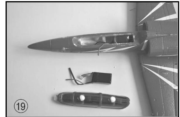
Fig. 19 - Locate the battery and canopy. Charge the battery according to the safety instructions before installing.
