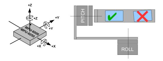
Skip Gyro calibration at startup - With this option, the board starts working immediately after powering it on, using the saved calibration data from last gyroscope calibration call.
