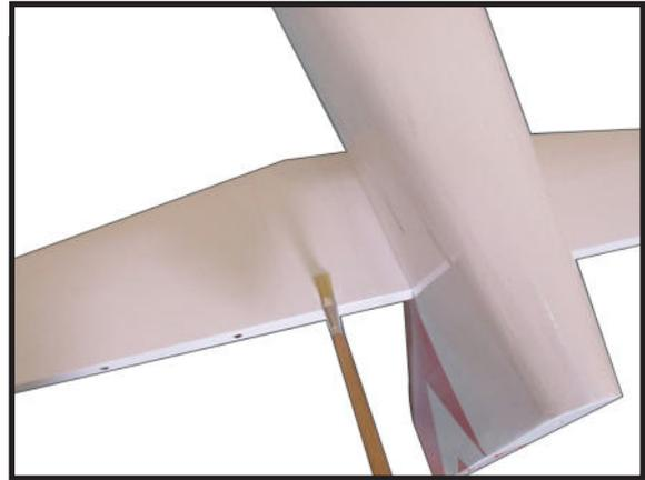
Once the alignment of the stabilizer has been verified, use a paper towel and isopropyl alcohol to remove any excess epoxy from the fuselage and stabilizer. Allow the epoxy to fully cure before proceeding.
