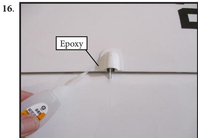
**INSTALLING ROBART LANDING GEAR**
