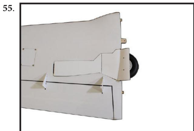
Continue Attaching the hinge to the cover and wing.
