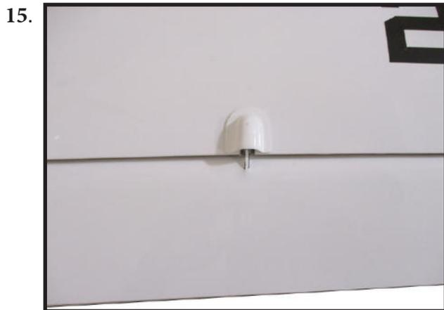
Use canopy glue to attach the cover to the wing. Use low-tack tape to keep the cover in position until the adhesive fully cures. Blue painters tape works well !
