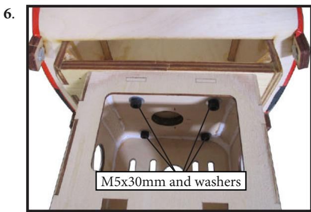
Then, use 5.2mm drill bit to enlarge the holes on the electric motor box.
