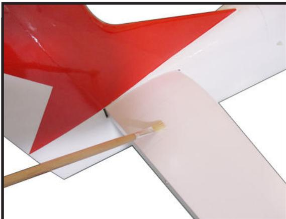
Carefully turn the model over and apply epoxy to the exposed wood on the bottom of the stabilizer. Slide the stabilizer back into position.
