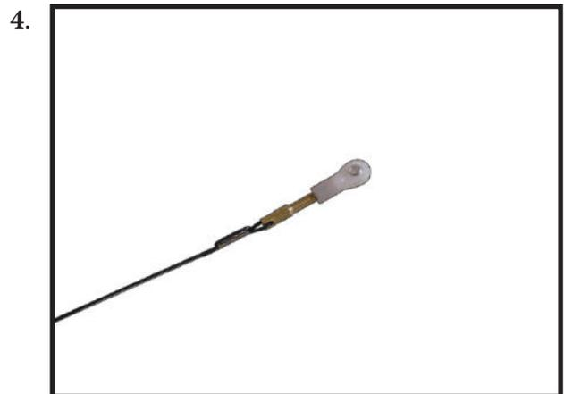
**RUDDER CABLE INSTALLATION**
