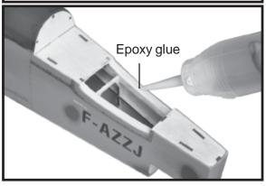
☐ 5. When you are sure that everything is aligned correctly, mix up a generous amount of 30 minute epoxy. Apply a thin layer to the top and bottom of the stabilizer mounting area and to the stabilizer mounting platform sides in the fuselage. Slide the stabilizer in place and re-align. Double check all of your measurements one more time before the
