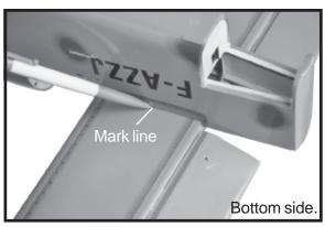
☐ 4. Remove the stabilizer. Using the lines you just drew as a guide, carefully remove the covering from between them using a modeling knife.
