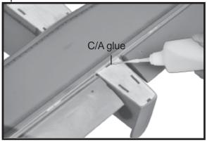
☐ 6. After the epoxy has fully cured, remov the masking tape or T-pins used to hold the stabilizer in place and carefully inspect the glue joints. Use more epoxy to fill in any gaps that were not filled previously and clean up the excess using a paper towel and rubbing alcohol.
