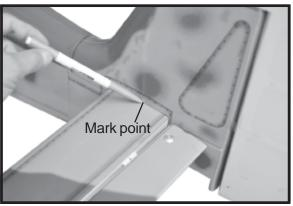
☐ 3. Mark the shape of the vertical on the left and right side on the rudder using a felt-tip pen.
