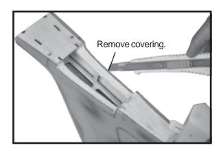
☐ Also carefully remove the covering from the horizontal fin as below the lines which you drew as same picture below.
