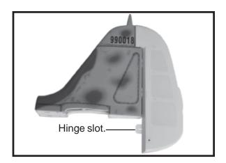
☐ 1) Using a modeling knife, remove the covering from the top of the fuselage and the covering from over the precut hinge slot cut into the lower rear portion of the fuselage This slot accepts the lower vertical.
