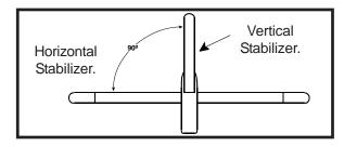
☐ 5. Put the vertical stabilizer back in place. Using a triangle, check to ensure that the vertical stabilizer is aligned 90 degree to the horizontal stabilizer.
