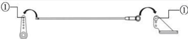
Control horn and servo arm locations for Ailerons
