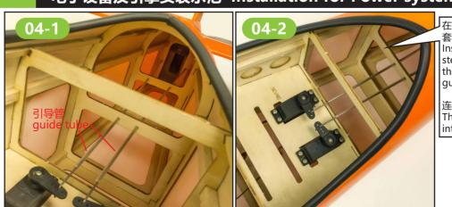
在机身内安装舵机,并把钢丝连杆插入机身内,钢丝套引导管,引导管用胶水固定在机身内。 Install the servos inside the fuselage, insert the steel wire linkage rod into the fuselage, insert the steel wire into the guide tube, and fix the guide tube inside the fuselage with glue.
