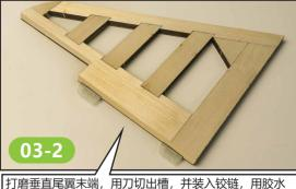
Grind the end of the vertical tail, and cut the groove with a knife, finally insert the hinge and fasten with
