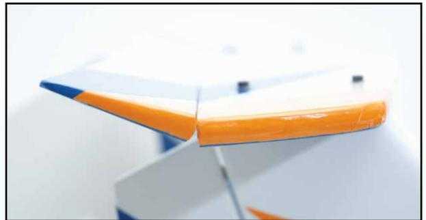
🇬🇧 Rudder: 26mm each way at base of rudder, with 10% exponential.
