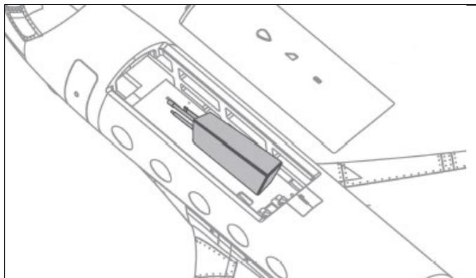
1. Before connecting the battery to the plane, power on the transmitter and ensure throttle lever in the lowest position.
