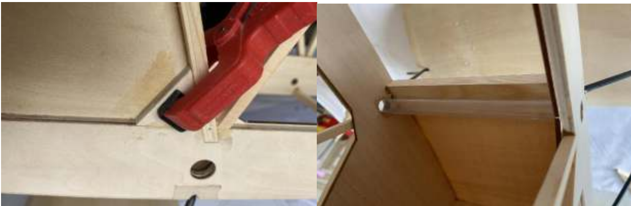
21) The pine block is attached to the nose to secure the cowling.
