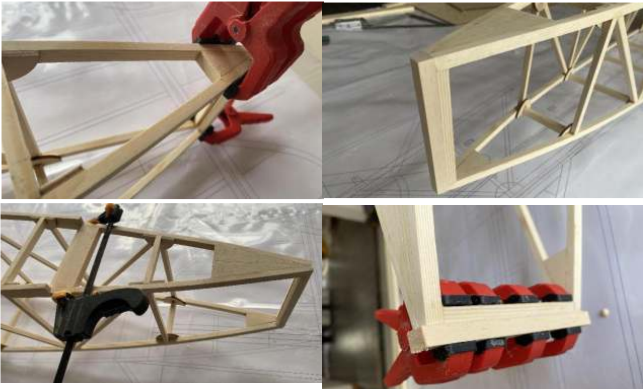
7) Glue 6X6MM pine strips as the tail diagonal supports.
