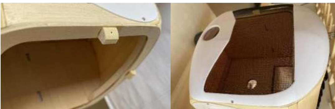
21) The pine block is attached to the nose to secure the cowling.
