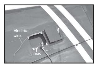
☐ 5. Instal servo tray with aileron servo into the wing as same as picture below.
