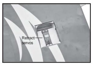
INSTALLING RETRACTABLE LANDING
