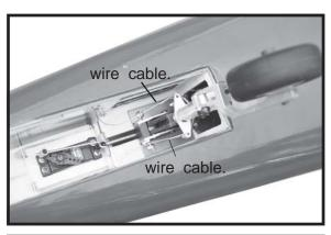
INSTALLING SERVO NOSE GEAR.
