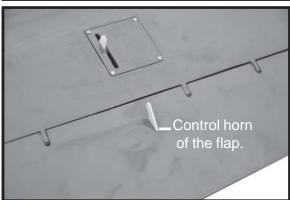
3.INSTALLING THE FLAP LINKAGES.
