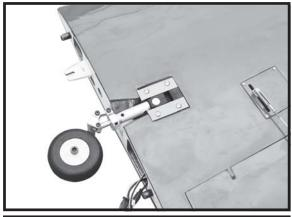
INSTALLING THE RETRACT PUSHROD.
