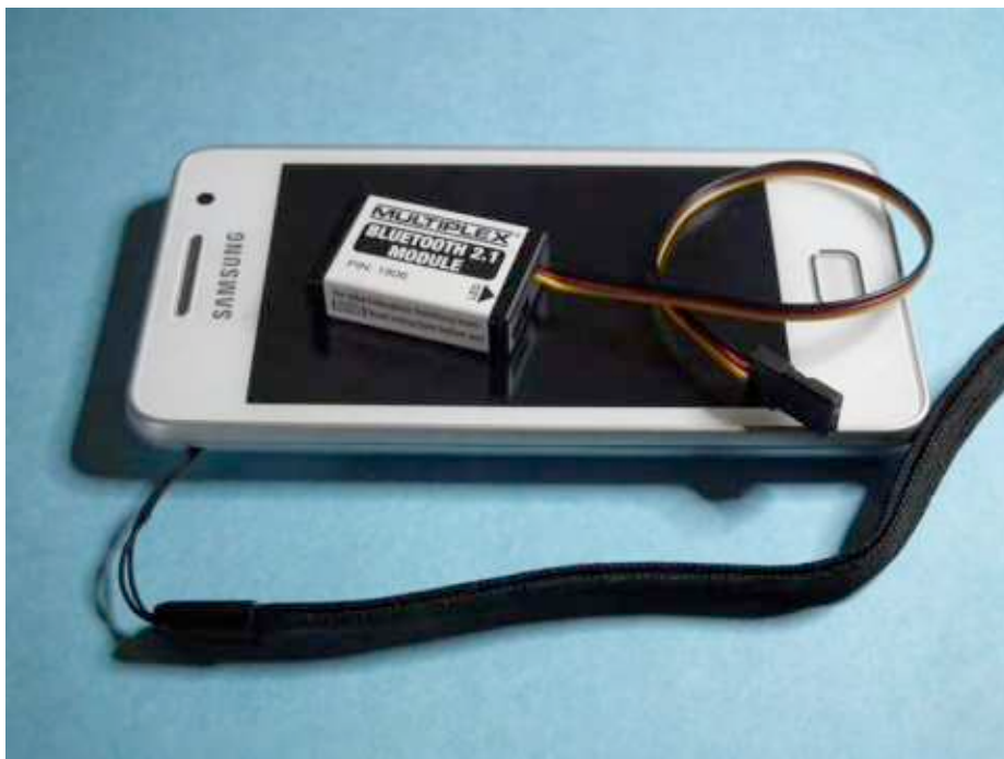
Figure 25: MPX Bluetooth adapter for WINGSTABI
