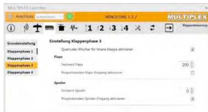
Figure 22: Flap phase settings
