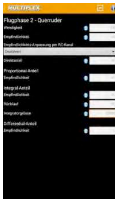
Figure 30: Gyro phase settings for WINGSTABI
