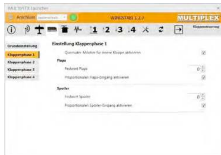
Figure 17: Alternative phase settings
