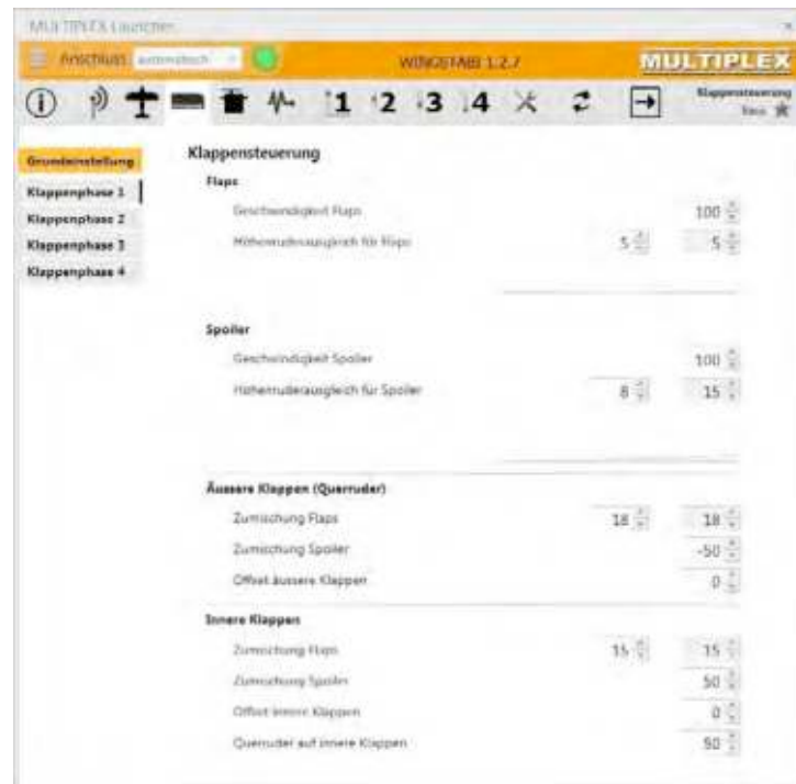
Figure20: Basic glider flap settings
