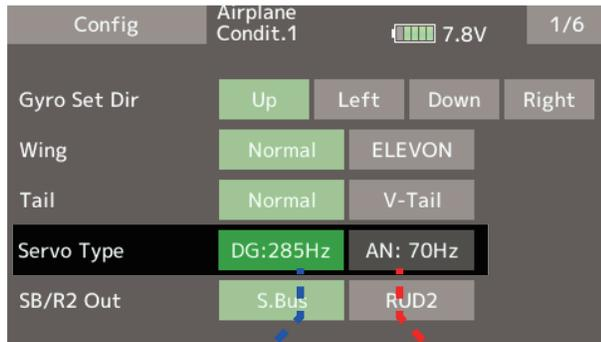
Select the servo type according to the servo to be used.
