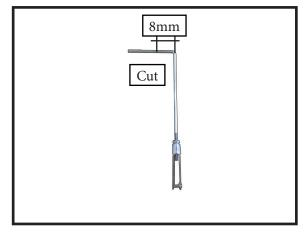
Make a 90-degree bend at the mark and cut off the excess wire leaving 8mm past the bend.
