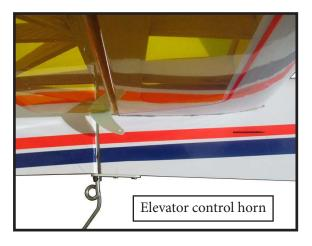
Thead one clevis and M2 lock nut on to each elevator control rod. Thead the horns on until they are flsh with the ends of the control rods.
