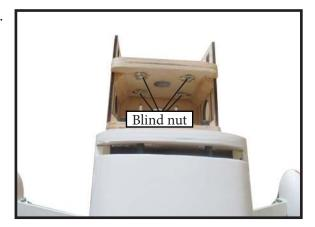
Attach the motor to the front of the electric motor box using four 3mm blind nut, four M3x20mm hex head bolts to secure the motor. Please see picture shown.
