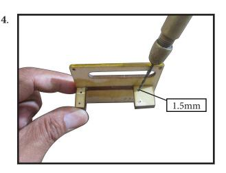
Apply 2-3 drops of thin C/A to each of the mounting holes. Allow the C/A to cure without using accelerator.
