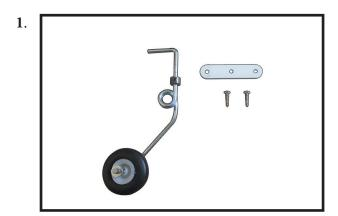
Test fit the tail gear to make sure that it fits properly. When you are happy with the fit, attach the tail gear using the two M3x20mm wood screws.
