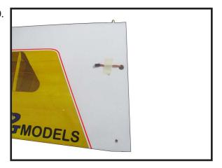
Apply 2-3 drops of thin C/A to each of the mounting aileron hatch mounting tabs in the wing. \*\*\*Allow the C/A to cure without using accelerator.\*\*\*
