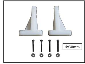
Use four 4x30mm head bolts and four 4mm washers to attach the engine mount rails to the fiewall. Tighten the screws . Make sure to use threadlock on the screws to help prevent them from vibrating loose.
