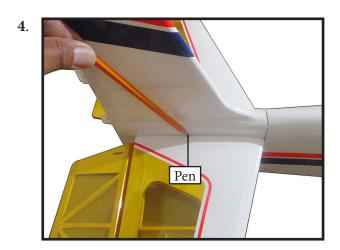
Remove the stabilizer. Using the lines you just drew as a guide, carefully remove the covering from between them using a modeling knife.
