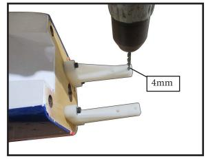
The fire wall has the location for the throttle pushrod tube (pre-drill).
