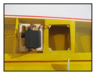
Set the aileron hatch in place and use a Phillips screw driver to install it with four wood screws.
