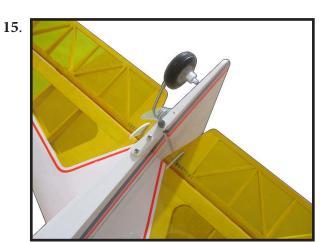
Hold the rudder in place and mark it where the music wire will enter. When you are happy with the fit, fill the hole with epoxy and use CA to glue in the rudder hinges.
