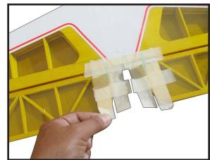
Using a modeling knife, carefully remove the covering at mounting slot of horizontal stabilizer (both side of fuselage).
