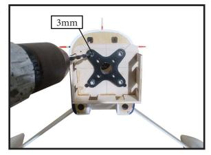
Then, use 3mm drill bit to enlarge the holes on the electric motor box.
