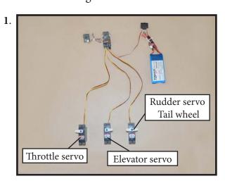
Secure the servos with the screws provided with your radio system.
