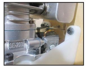
Attach throttle pushrod to the carburetor throttle arm with the ball link.
