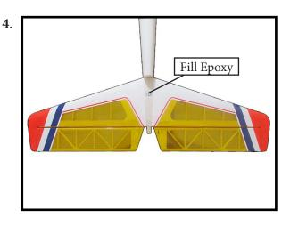
Slide the vertical stabilizer back in place. Using a triangle, check to ensure that the vertical stabilizer is aligned 90° to the horizontal stabilizer.
