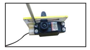
6) Apply 1-2 drops of thin C/A to each of the mounting tabs. Allow the C/A to cure without using accelerator.
