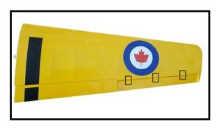
Note: Work the aileron up and down several times to "work in" the hinges and check for proper movement.
