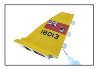
1) While holding the vertical stabilizer firmly in place, use a pen and draw a line on each side of the vertical stabilizer where it meets the top of the fuselage.
