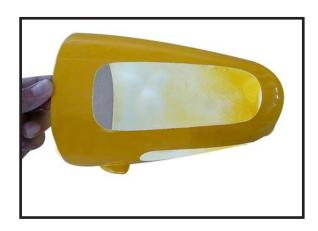
1) Tape the cowl to the fuselage using low-tack tape.
