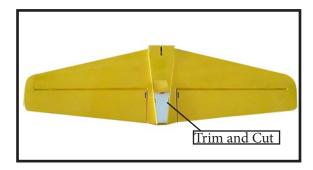
When cutting through the covering to remove it, cut with only enough pressure to only cut through the covering itself. Cutting into the balsa structure may weaken it.
