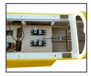
RUDDER PUSHROD HORN INSTALLATION.
