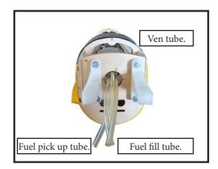
9) Connect the lines from the tank to the engine and muffl. Th vent line will connectto the muffl and the line from the clunk tothe carburetor.
