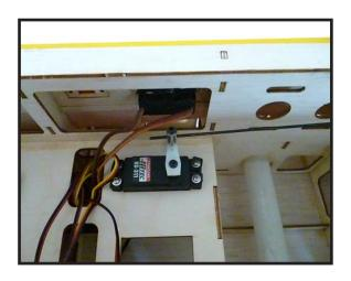
9) Move the throttle stick to the closed position and move the carburetor to closed. Use a 2.5mm hex wrench to tighten the screw that secures the throttle pushrod wire. Make sure to use threadlock on the screw so it does not vibrate loose.
