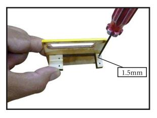
3) Apply 2-3 drops of thin C/A to each of the mounting holes. Allow the C/A to cure without using accelerator.
