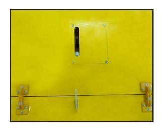
INSTALLING THE FLAP PUSHROD.
