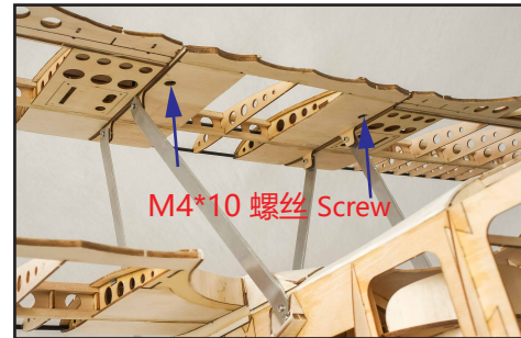
机翼支架安装图示 Wing's bracket installation show
