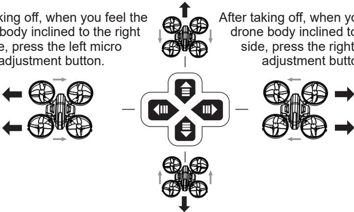
After taking off .when you feel the drone body inclined ahead, press the backward micro adjustment button.
