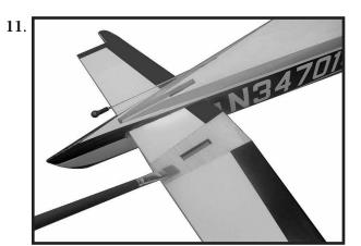
Carefully turn the model over and apply epoxy to the exposed wood on the bottom of the stabilizer. Slide the stabilizer back into position.
