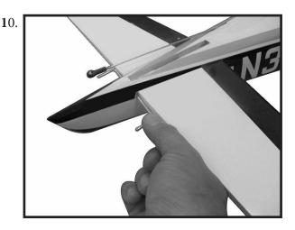
Slide the stabilizer partially into the fuselage so the wood at the center is exposed. Mix 1/2 ounce (15ml) of 30-minute epoxy. Use an epoxy brush to apply the epoxy to the exposed wood on the top of the stabilizer.
