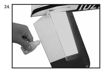
Gently pull on the fixed and moving surface to make sure the hinges are glued securely. If not, reapply thin CA to any hinges that are found loose.
