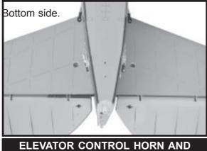
Elevator control horn install as same as the way of aileron control horn. Please see pictures below.
