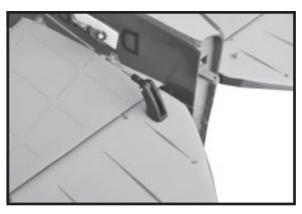
Plastic parts of elevator pushrod.
