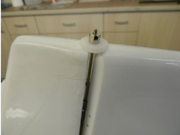
27-) Then, cut the steel wire flush with the wheel collar.
