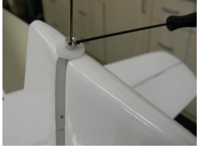
26-) From the top, slide the plastic round disc and secure it with the small wheel collar.
