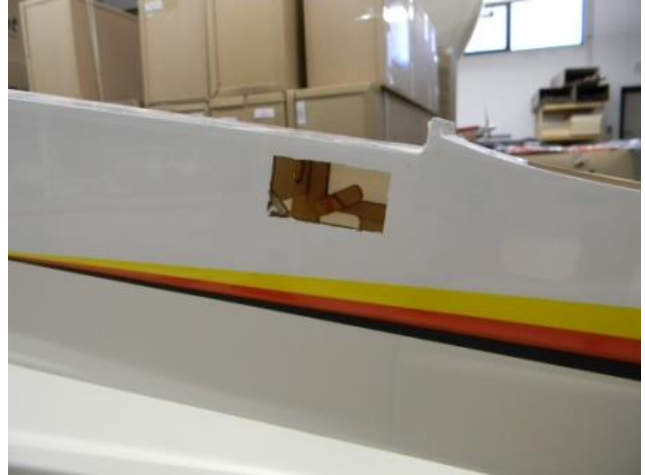
28-) On the rear Left side of the fuselage, in front of the stab saddle, open the elevator servo cavity by cutting the covering film.
