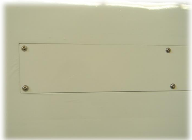
62-) Secure the bottom spoiler cover at each corners and center with the supplied wood screws.
