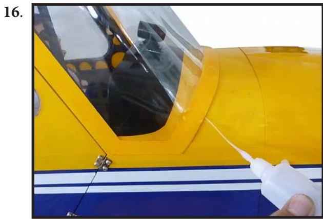
Epoxy canopy onto the fuselage. Trace around the canopy and onto the fuselage using a epoxy.
