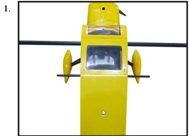
Attach the aluminiu, thube into fuselage.
