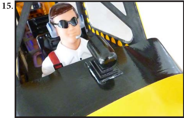
Epoxy canopy onto the fuselage. Trace around the canopy and onto the fuselage using a epoxy.
