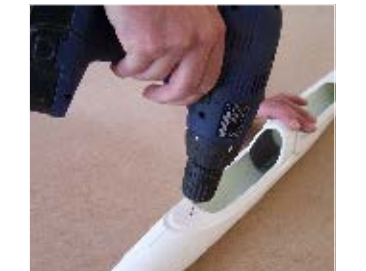
75. ...vyvrtáme otvor Ø2,2mm... ... drill hole Ø 2.2 mm ...
