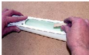
104. ...a desku vlepíme do trupu ... and glue plate to the fuselage.
