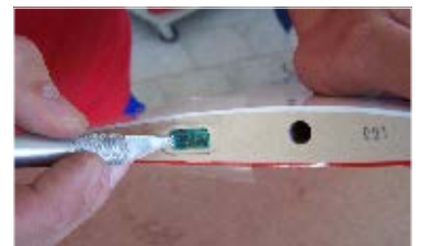
64. ...v pásce vyřízneme otvor pro protikus konektoru... ... cut hole in the tape for complemented connector ...
