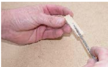
103. Desku natřeme lepidlem... Put glue on the plate surface ...
