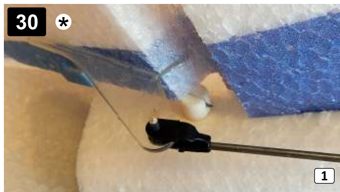
Ocelová struna zacvaknuta v drážce. String is inside the slot.
