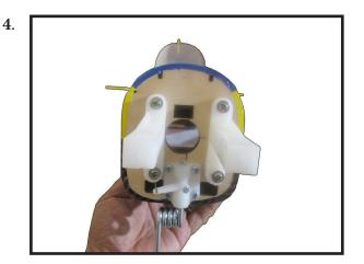
Position the engine with the drive washer (145mm) forward of the firewall as shown.
