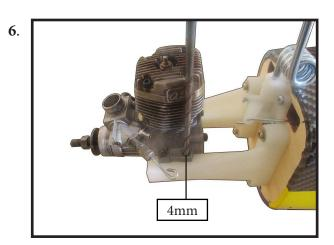
Use a drill to drill the four holes in the engine mount rails.
