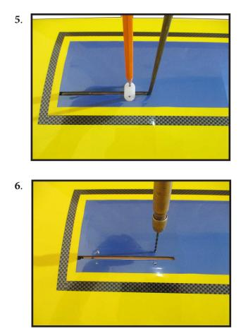
Remove the two straps and the gear wire. Drill four 3/32" pilot holes into the wing for the wood screws.
