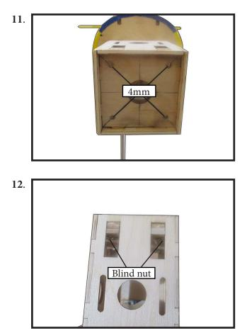
Attach the motor to the front of the electric motor box using four 3mm blind nut, four M3x20mm hex head bolts to secure the motor. Please see picture shown.
