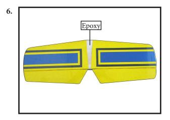
When you are sure that everything is aligned correctly, mix up a generous amount of 30 Minute Epoxy. Apply a thin layer to the top and bottom of the stabilizer mounting area and to the stabilizer mounting platform sides in the fuselage. Slide the stabilizer in place and realign. Double check all of your measurements once more before the epoxy cures. Hold the stabilizer in place with T-pins or masking tape and remove any excess epoxy using a paper towel and rubbing alcohol.
