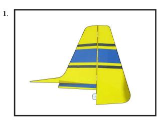
Using a modeling knife, remove the covering from over the precut hinge slot cut into the lower rear portion of the fuselage. This slot accepts the lower rudder hinge.
