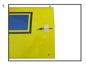
Reinstall the servo into the servo mount and secure the servo inplace using the wood screws provided with you radio system.
