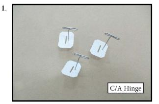
Remove each hinge from the wing panel and aileron and place a T-pin in the center of each hinge. Slide each hinge into the wing panel until the T-pin is snug against the wing panel. This will help ensure an equal amount of hinge is on either side of the hinge line when the aileron is mounted to the aileron.
