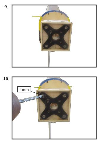
Then, use 4mm drill bit to enlarge the holes on the electric motor box.
