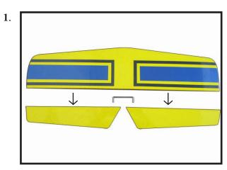
Carefully remove the elevator from one of the horizontal stabilizer panels. Note the position of the hinges.
