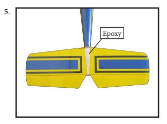
Slide the vertical stabilizer back inplace. Using a triangle, check to ensure that the vertical stabilizer is aligned 90° to the horizontal stabilizer.
