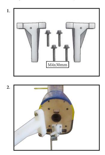
Use four 4x30mm head bolts and four 4mm washers to attach the engine mount rails to the firewall. Tighten the screws .Make sure to use threadlock on the screws to help prevent them from vibrating loose.
