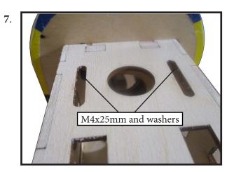
Attach the motor mount to the front of the electric motor box using four 4mm blind nut, four M4x25mm hex head bolts to secure the motor. Please see picture shown.
