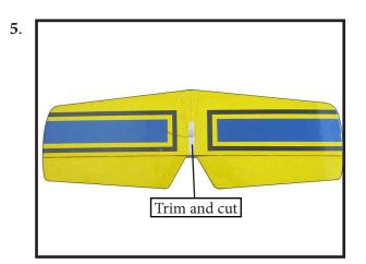
/ <u>When cutting through the covering</u> to remove it, cut with only enough pressure to only cut through the covering itself. Cutting into the balsa structure may weaken it.
